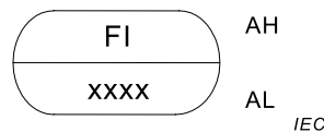
Figure 11 – Example of flow measurement with indication in the CCR and high and low alarm
